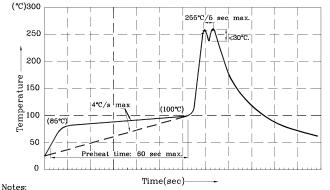
I.Recommend pre-heat temperature of 105°C or less (as measured with a thermocouple attached to the LED pins) prior to immersion in the solder wave with a maximum solder bath temperature of  $260^{\circ}$ C 2.Peak wave soldering temperature between  $245^{\circ}$ C ~  $255^{\circ}$ C for 3 sec
