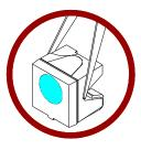
2. Do not directly touch or handle the silicone lens surface. It may damage the internal circuitry.
