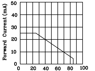
Ambient Temperature T_A ( ^\circ\text{C} ) FORWARD CURRENT DERATING CURVE
